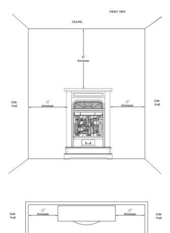
Figure 4-Minimum Clearance to Wall
